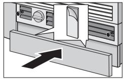
■ Remove the foil from the adhesive strips.
